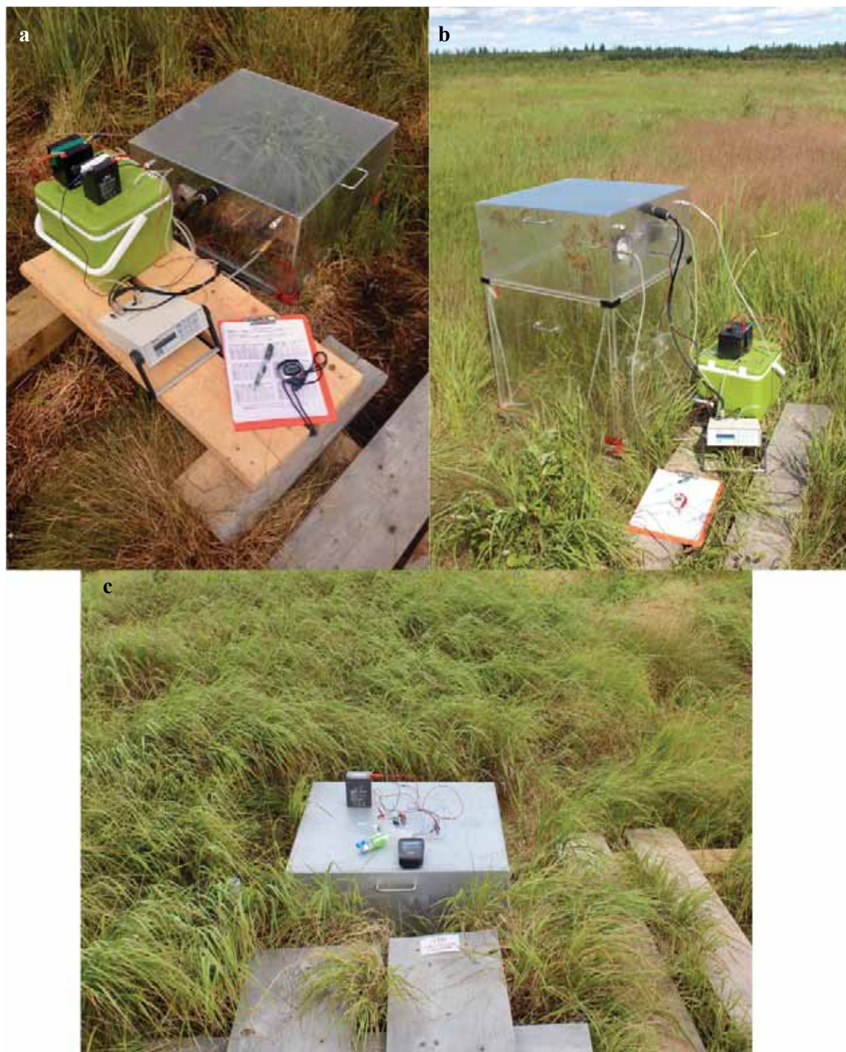
Figure A3 Chamber measurements of (a,b) \text{CO}_2 and (c) \text{CH}_4 . These pictures represent measurements in the wet section, where species taller than the chamber (e.g. S.cyp and B.syz ) used a clear extension (b), which was also adapted to \text{CH}_4 fluxes measurements.
