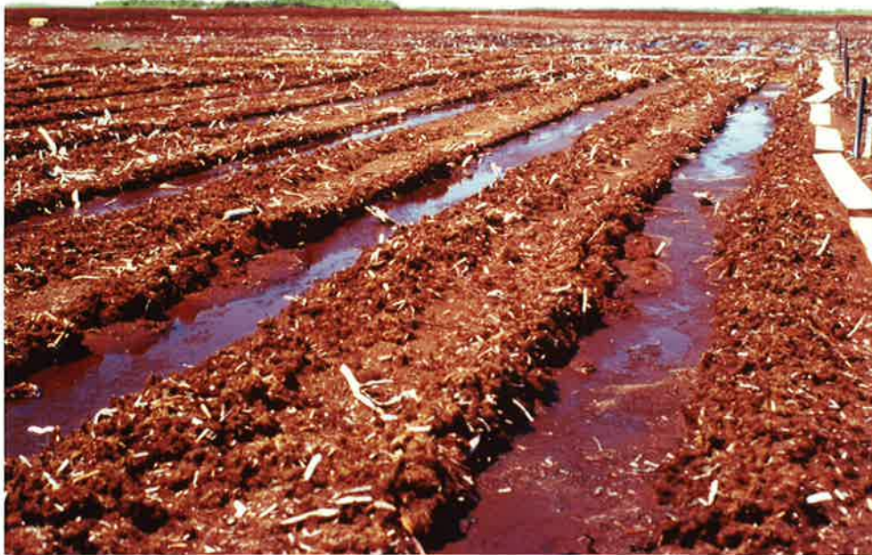
Plate 1. Example of a plot with irregular microtopography at the Maisonnette experimental site. The alternating ridges and depressions were made in the spring of 1993 by the passage of an excavator when the ground was still partly frozen.
