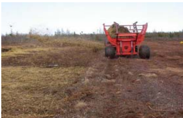
5e. Straw spreading with a lateral straw spreader.
