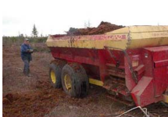
5d. Sphagnum introduction with a lateral manure spreader.
