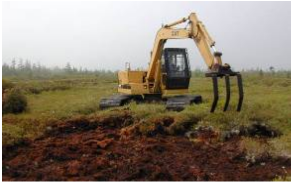
5a. Vegetation harvest with the help of an excavator equipped with a mechanical fork.
