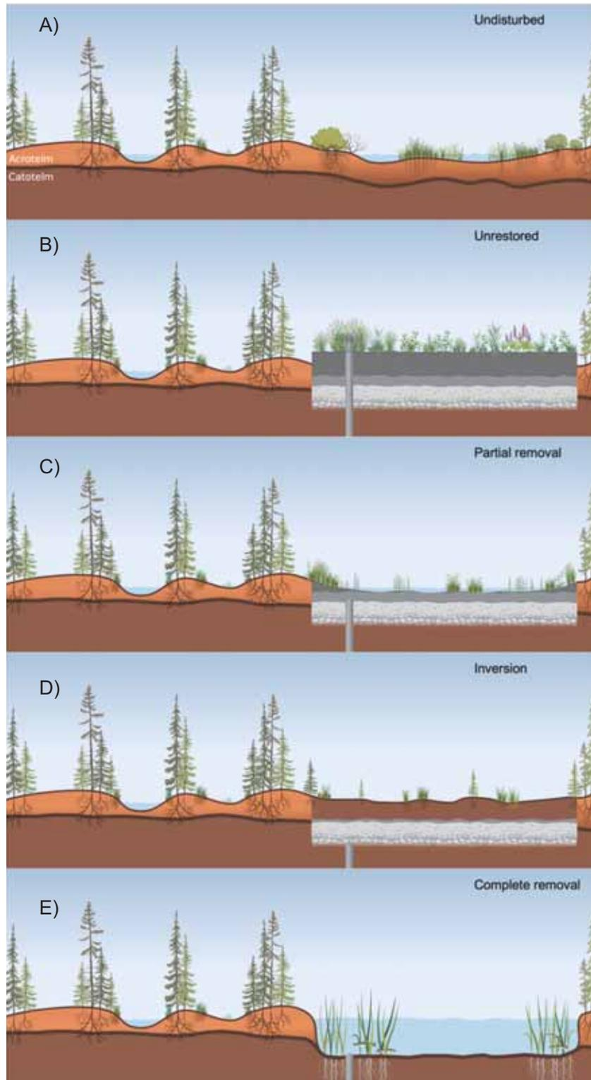
*Figure 0.4 Schematic cross section of A) a pristine peatland before disturbance, in comparison to the B) unrestored peatland disturbed by an decommissioned/ abandoned in situ oil sands well pad, and peatlands restored via C) the partial removal of the mineral fill, via D) the inversion of the mineral fill and the underlying peat, and via E) the complete removal of the former in situ well pad, where a shallow open water area formed instead.*
