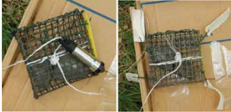
Figure 16. Cotton strips were installed in vernal pools and maintained few centimeters above the soil surface (picture on the right). Mini-Diver probes were used to measured water levels and temperature in each pool (picture on the left).
