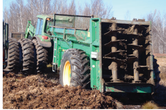
Figure 4. Apron box manure spreader with vertical beaters.
