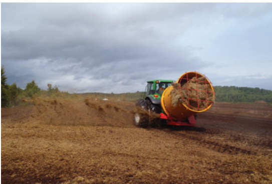
Figure 10. Rear-loading side-discharge mulcher.
