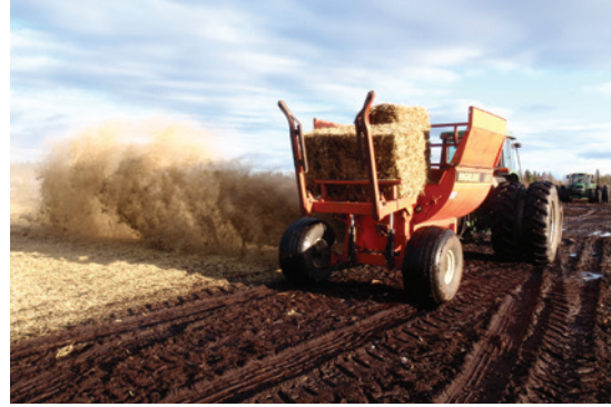
Figure 9. Side-discharge mulcher (rear view).
