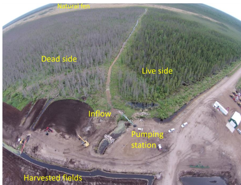
Figure 1. Drone image of the live side to the east and dead side to the west. As well, the pumping station where the water was routed from the fields and into the drainage ditch.
