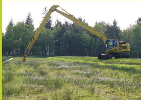
**Figure 33.** Long-reach excavator, equipped with a weed cutter, working from the embankment.
