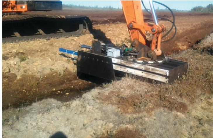
**Figure 40.** Device used in Canada for block-cut peat extraction. Tests have shown that this equipment could also be used to harvest *Sphagnum*.
