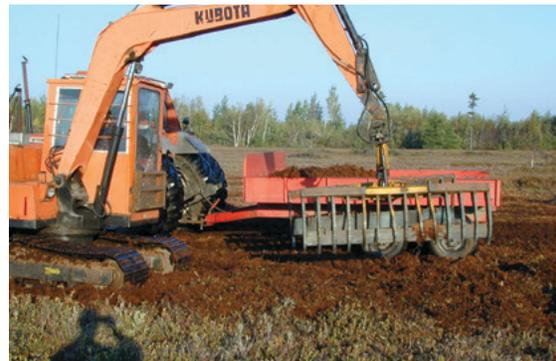
**Figure 23.** Collecting material after the rotary tiller has passed.
