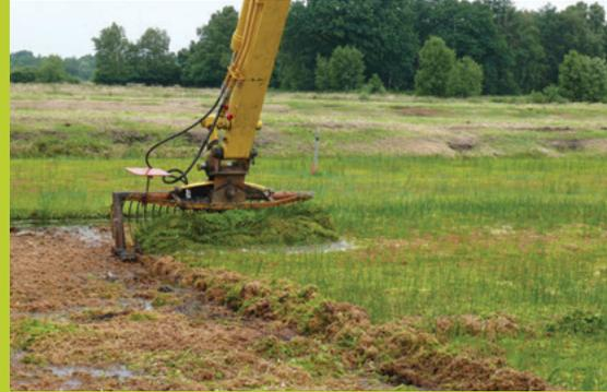
**Figure 37.** Excavator with a weed cutter at the end of its boom being used to cut *Sphagnum*.
