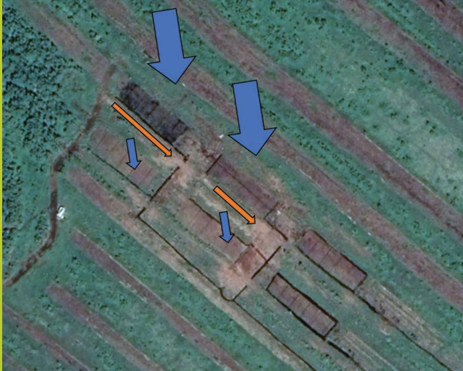
**Figure 14.** Interception of natural water flow by reservoir canals. Blue arrows indicate natural water flow intensity, and orange arrows show where the flow is intercepted by canals (image: 2022 CNES/Airbus).
