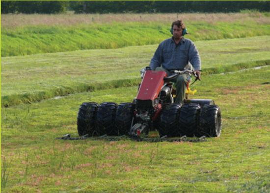
**Figure 32.** Single-axle mower with cutter bar being used to control the common rush.
