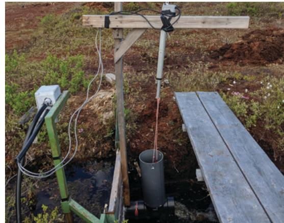
**Figure 19.** Mobile dam operating with a sonar that measures the water level in the reservoir canal, and with a linear actuator and a float (in the grey pipe) to open the dam valve.
