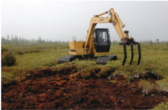
**Figure 20.** Harvesting plant material in a former block extraction site using a crawler excavator with a fork attachment.
