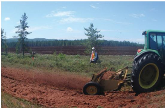
**Figure 22.** Shredding plant material with a rotary tiller, in an undisturbed peatland.
