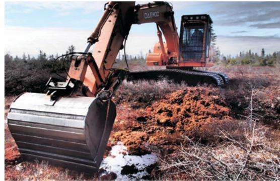
**Figure 21.** Harvesting plant material in a former block extraction site using an excavator with a bucket to scrape the thawed surface layer of *Sphagnum* in spring.
