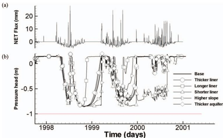
Figure 8. Transient case 1. (a) NET Flux (mm) and (b) Transient pressure response to daily climate inputs (rain, snowmelt, evaporation and transpiration) and using Liner II, Aquifer II properties.
